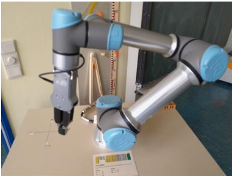
Figure 4-1: Examination structure of UR5
