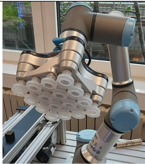
Suction lifter from the company OnRobot
