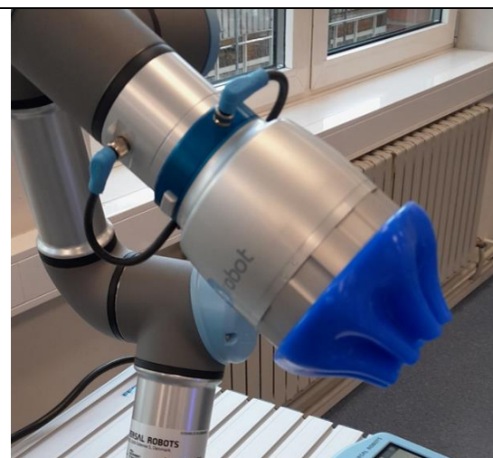
„Softgripper“ from the company OnRobot
