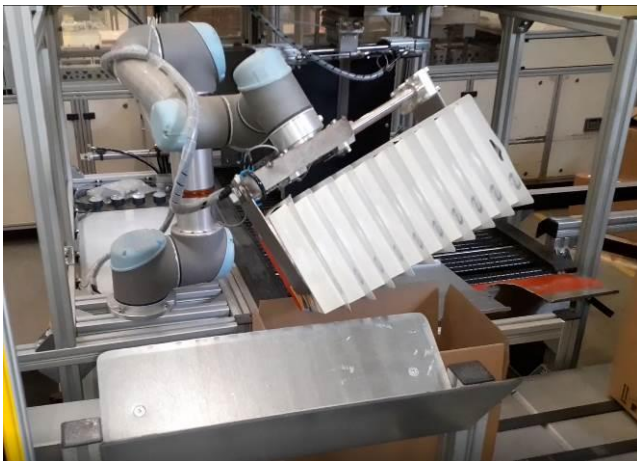
Figure 2-3: Mechanical centring in the packaging process
