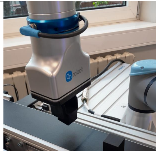
Parallelgripper from the company OnRobot
