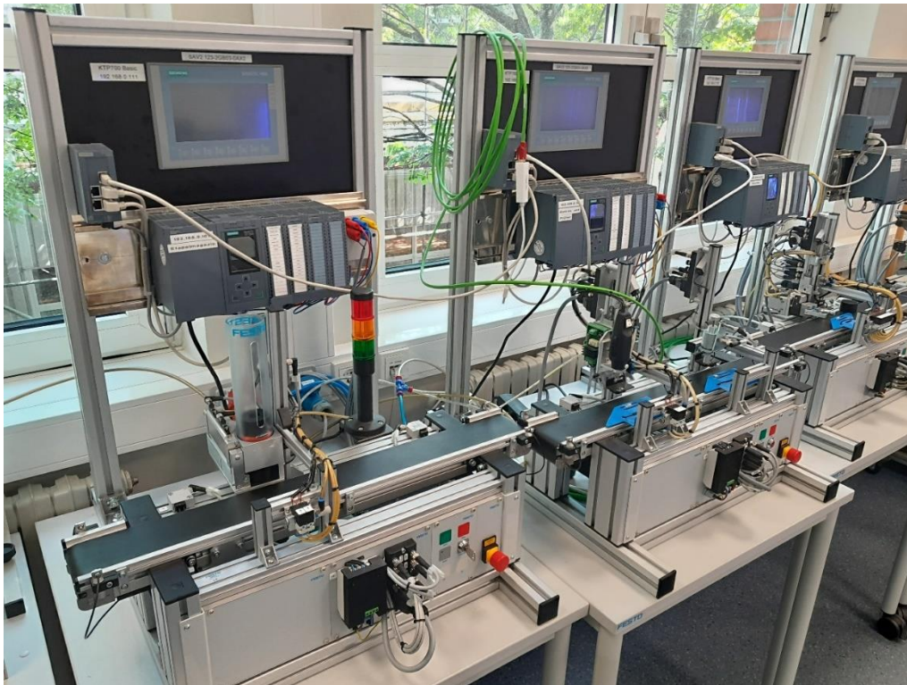
Figure 5-2 FESTO Didactics MPS conveyor system with expansion modules (from left: 1. stacking magazine, 2. drilling and depth testing, 3. turning components, 4. RFID reading, writing and ejection)
