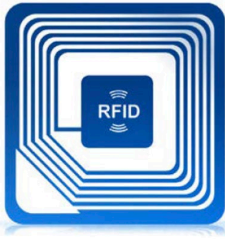
Figure 9: This is an RFID tag, and the pattern around it is the antenna (graphics courtesy of FESTO).
